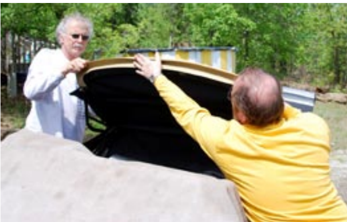
Tissue paper from the new top covers the trunk area of a Spider as David Simmons and James Perlingiere concentrate on their job.
